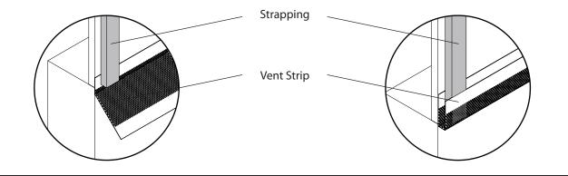
PAINT ALL FIELD CUTS. Seal all field cuts with Cape Cod Siding touchup paint. Scratches & any other damage caused by installation must be repaired. Do not apply touchup paint to the factory painted surface of the siding as color variation can occur.
